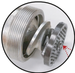
ASSEMBLE ORDER: WORM, KNIFE AND PLATE
