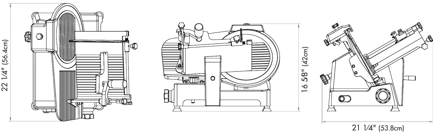
Controls: Manual slice thickness knob, push button on/off, attached blade sharpener
